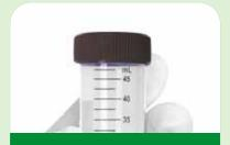
Screw the cap on the tube tightly so it doesn't leak.
